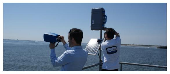
WISP Stations are installed in 6 countries to analyse Chlorophyll-a Water Insight installed six WISP Stations to analyse water quality, focusing on Chlorophyll-a, total suspended matter, coefficient of downwelling irradiance, cyanobacteria pigment and colored dissolved organic matter.<u>*Read more...*</u>
