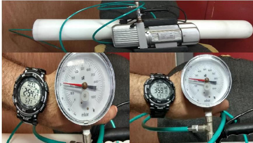
Figure 9: The ASP housing internal pressure test
