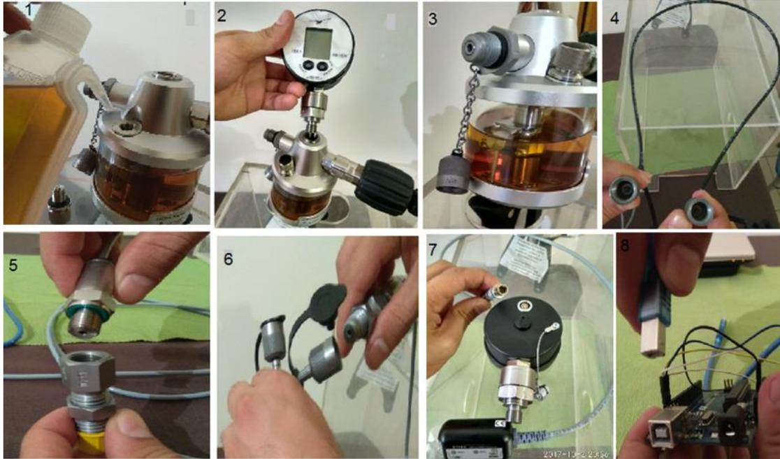
Figure 7: The ASP pressure sensor calibration procedure
