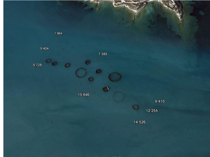
Location of sediment traps surrounding the fish farm. The average suspended sediment collected during a two-week period is illustrated at each site.
